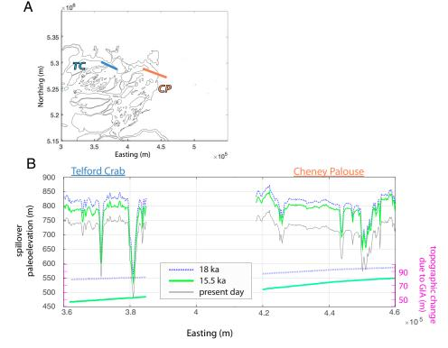
Fig. 4. (A) Transect for Cheney-Palouse (CP; orange) and Telford-Crab Creek (TC; blue). (B) Paleoelevation profiles (Left y-axis) and topographic change due to GIA relative to present day (Right y-axis) for 18 ka (dashed blue), 15.5 ka (green), and present day (gray) across spillover transects in A: TC (blue) and CP (orange), UTM zone 11.
